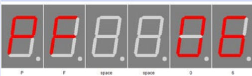
StandBy (Powersave) Finish Hour - Endstunde
