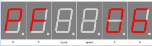
StandBy (Powersave) Finish Hour - Endstunde
