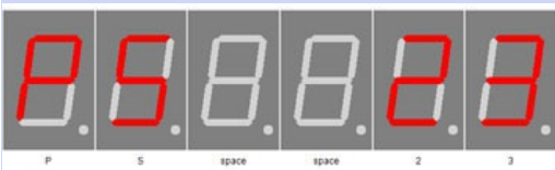
StandBy (Powersave) Start Hour
