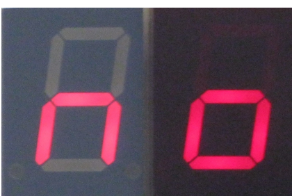
Figure 3: SA08-11SRWA left without and right with contrast pane with front light.
