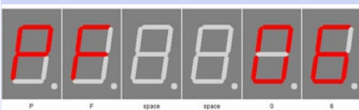
StandBy (Powersave) Finish Hour - Endstunde
