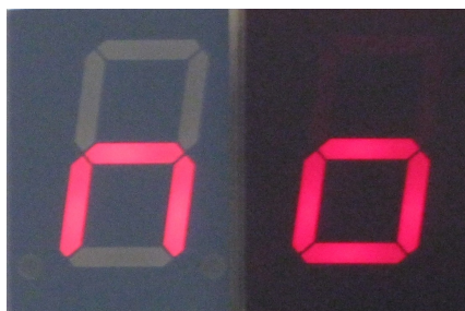
Figure 7: SA08-11SRWA left without and right with contrast pane without front light.
