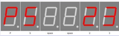
StandBy (Powersave) Start Hour
