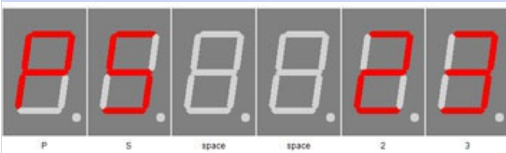
StandBy (Powersave) Start Hour
