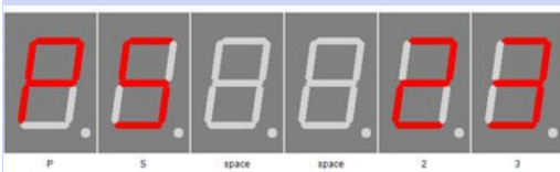
StandBy (Powersave) Start Hour
