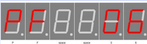
StandBy (Powersave) Finish Hour - Endstunde
