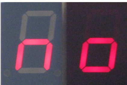
Figure 5: SA08-11SRWA left without and right with contrast pane without back light.
