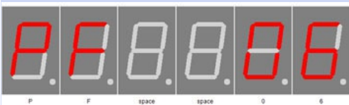
StandBy (Powersave) Finish Hour - Endstunde
