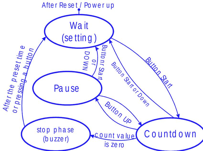
Figure - Abbildung 1 State diagram countdown mode
