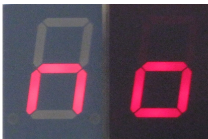
Figure 6: SA08-11SRWA left without and right with contrast pane without back light.
