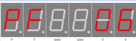
StandBy (Powersave) Finish Hour - Endstunde
