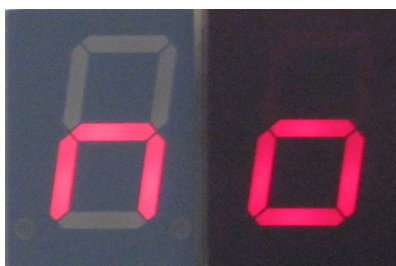
Figure 32: SA08-11SRWA left without and right with contrast pane without front light.
