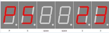
StandBy (Powersave) Start Hour
