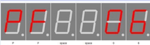
StandBy (Powersave) Finish Hour - Endstunde
