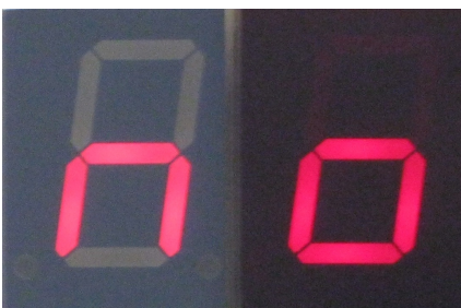
Figure 16: SA08-11SRWA left without and right with contrast pane without back light.
